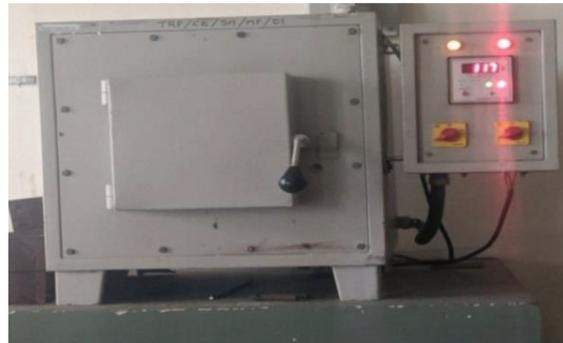
FIGURE 1: Heat treatment by muffle furnace KSM-0012.
