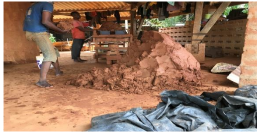
Fig. 5. Clay preparation and brick production
