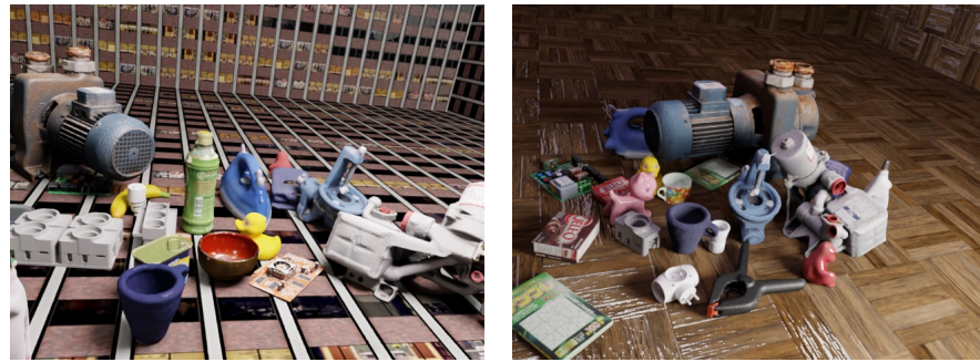
Figure 5. Photorealistic synthetic images generated using BlenderProc4BOP [18] with some of the 3D models used in our experiments, where other 3D models of different data sets, such as LINEMOD [15] or T-LESS [36], were used as distractors.
