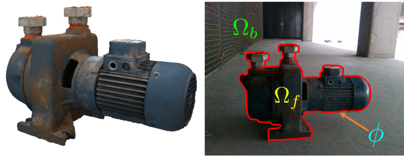
Figure 6. Left Image: 3D model. Right Image: Initialization of the tracking method by projecting the 3D model on the 2D image captured by the camera for a certain pose G (see Equation (4)). The projected object contour determines the background, \Omega_b , and the foreground, \Omega_f .
