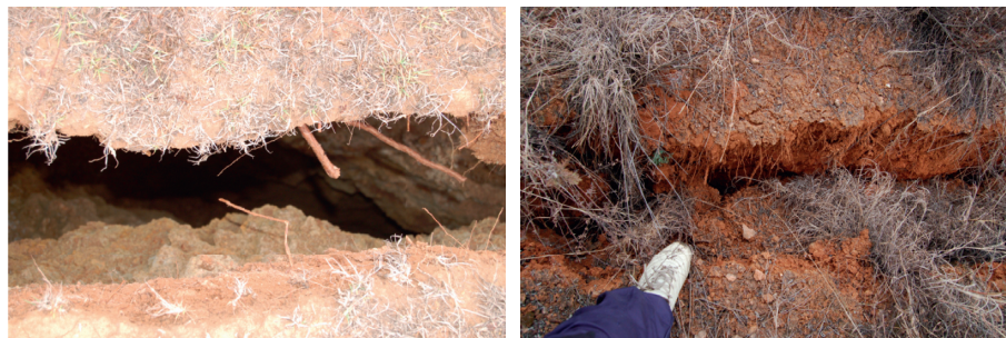
FIGURE 15: Point 4: surface soil fractures above the working face.
