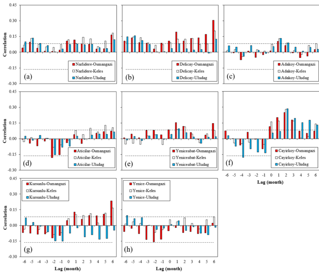
Figure 4. Cross-correlation diagram indicating the lagged interaction of SPI in the Osmangazi, Keles, and Uludag stations with the SGL in (a) Narlidere, (b) Delicay, (c) Adakoy, (d) Aticilar, (e) Yeniceabat, (f) Cayirkoy, (g) Kursunlu, and (h) Yenice.
