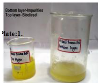
Plate 7. Alkali Trans-esterification process for Sesame oil
