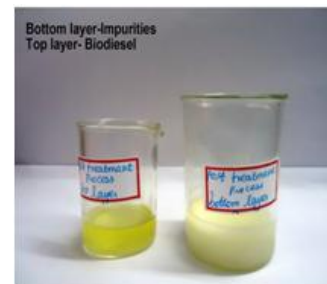
Plate 8. Post treatment process for Sesame oil
