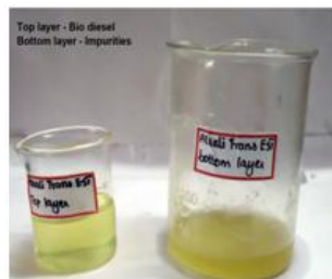
Plate 2. Alkali Trans-esterification process for sunflower oil
