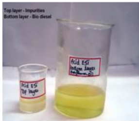
Plate 1. Acid catalyzed Trans-esterification process for sunflower oil
