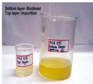
Plate 6. Acid catalyzed Trans-esterification process for Sesame oil
