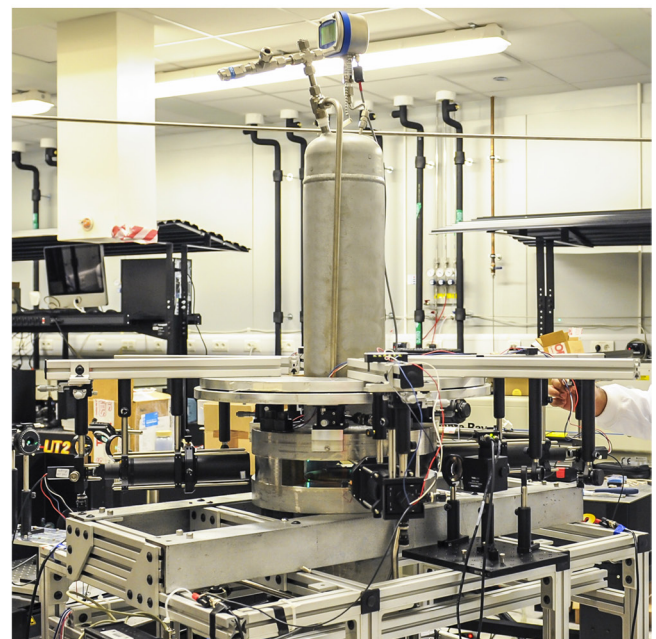
Figure 3. Schematic of pressure vessel with scattered light collection optics (top) and photograph of the experimental setup (bottom). Reprinted from [28]. Copyright 2017, with permission from Elsevier.
