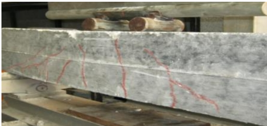
Fig. 2. Pre-cracks are marked
