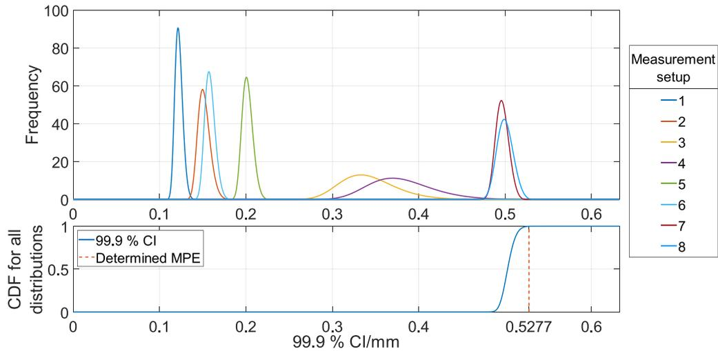
**Figure 13.** Determination of a final MPE following additional measurement in measurement setup 8: top; distribution of the maximal endpoint of the 99.9% CIs from bootstrapped data for each measurement setup and bottom; product CDF, with the 99.9% quantile highlighted.
