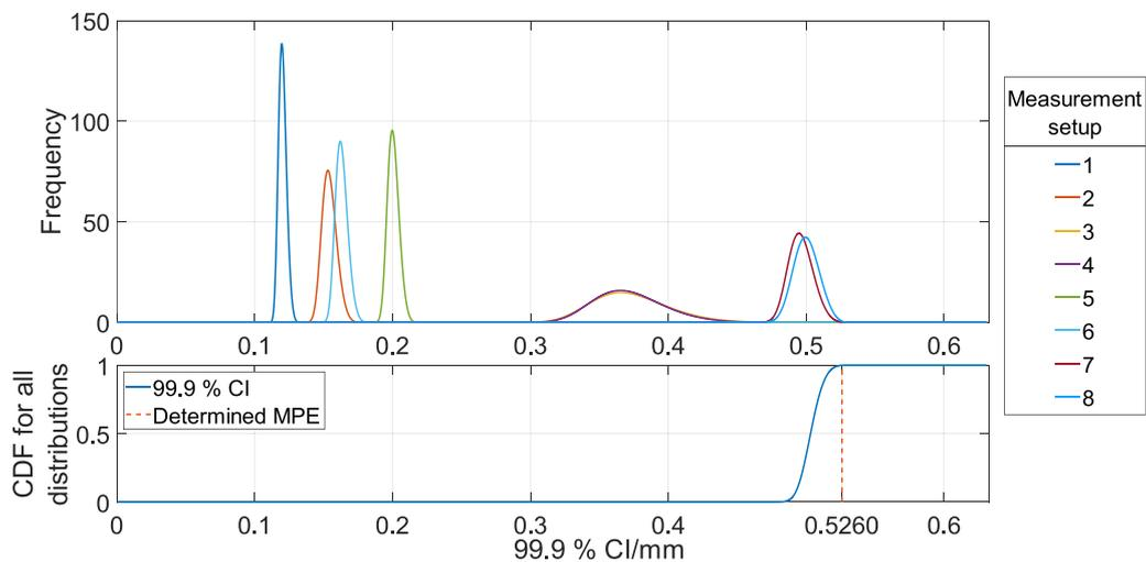
**Figure 14.** Brute-force validation of the data-efficient determined MPE, using 1000 measurements for each measurement setup: top; distribution of the maximal endpoint of the 99.9% CIs from bootstrapped data for each measurement setup and bottom; product CDF, with the 99.9% quantile highlighted.
