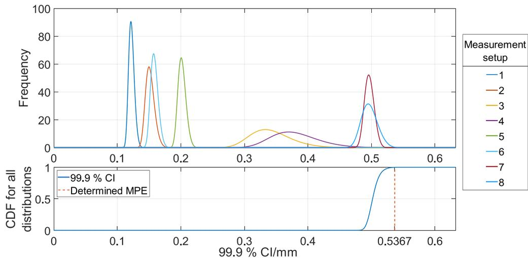
**Figure 12.** First-pass calculation of the MPE: top; distribution of the maximal endpoint of the 99.9% CIs from bootstrapped data for each measurement setup and bottom; product CDF, with the 99.9% quantile highlighted.
