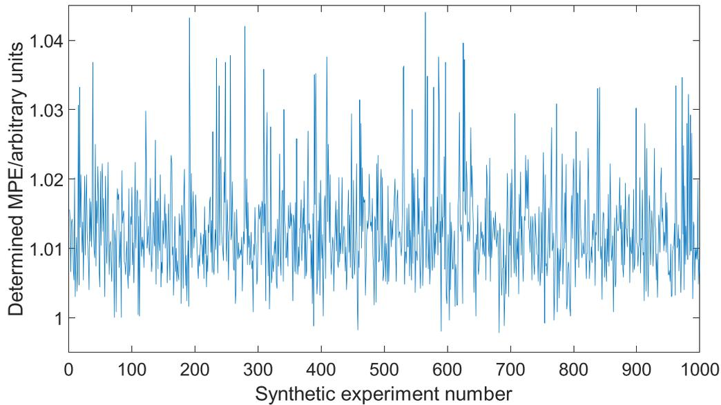
**Figure 7.** The efficient determined MPE over 1000 repeat experiments, where the true value is 1. Values greater than one represent the efficient MPE being larger than the true MPE (i.e. overestimation), with values less than one representing the converse.
