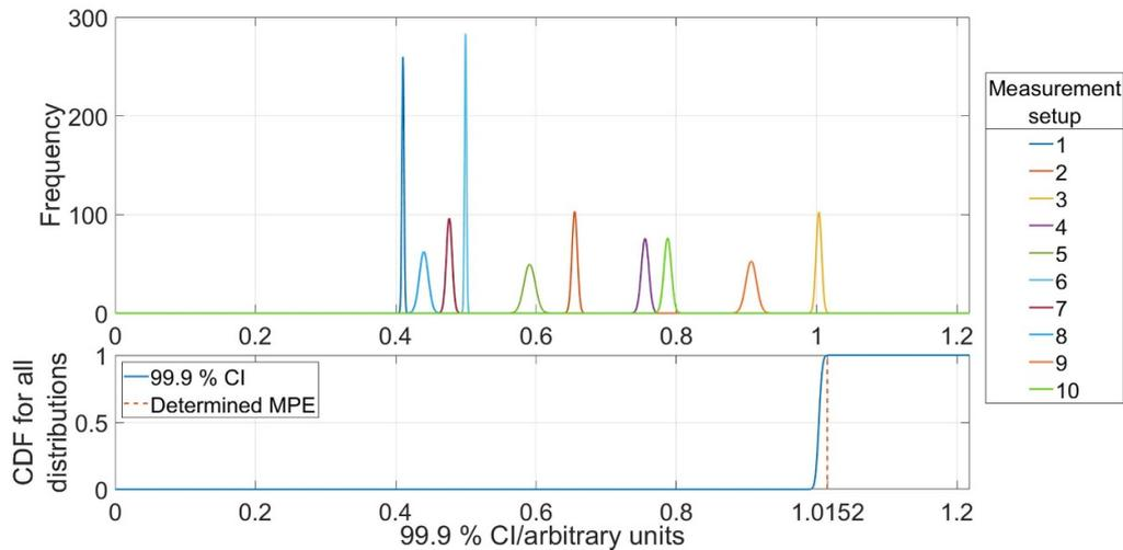
**Figure 6.** First-pass calculation of the MPE: top; distribution of the maximal endpoint of the 99.9% CIs from bootstrapped data for each measurement setup; and bottom; product CDF, with the 99.9% quantile highlighted.
