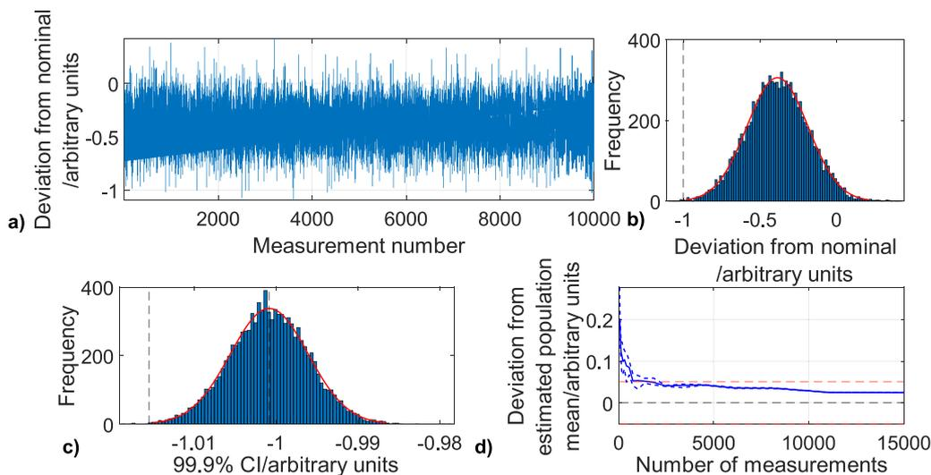
**Figure 5.** Determination of the of repeat measurements required for each other measurement setup using measurement setup 3: (a) deviation from nominal value for 10 000 measurements; (b) normal distribution fitted to deviations; (c) PDF of the maximal endpoint of the 99.9% CI for each bootstrap, with a normal distribution fitted to infer the maximal endpoint of the 99.9% CI of the population; and (d) convergence of the setup-specific MPE to the estimated maximal endpoint of the 99.9% CI.
