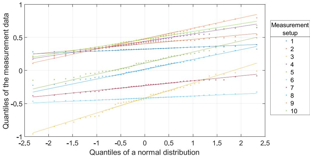
**Figure 4.** *Q*–*Q* plots of the 1st 50 synthetic measurements for a normal distribution fitted to each dataset.
