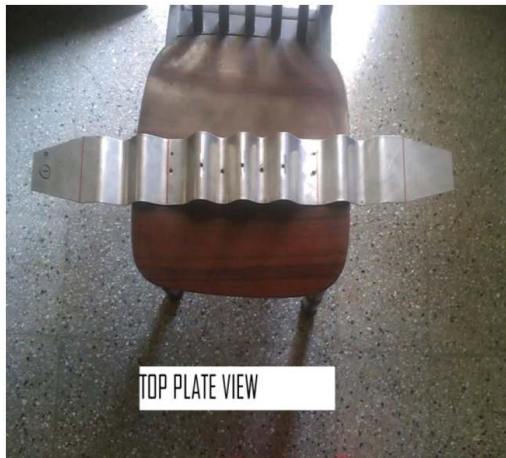
Fig. 5 Photographic view of top view of top corrugated plate
