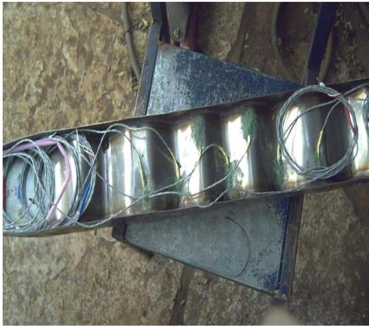
Fig. 4. Photographic view of fixing thermocouples of middle corrugated plate
