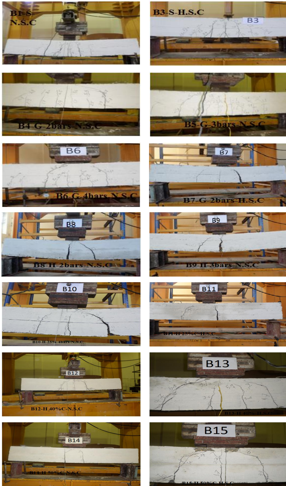
Fig. 6. Crack patterns of the tested beams
