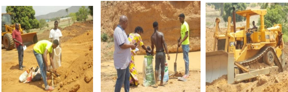
Fig. 10. Samples collection at Dabi site where Dantata and Sawoe Construction Company is using for Gwagwalada-Kwali road construction
