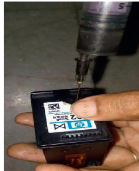
FIGURE 8: HP 302 cartridge filled with nanoparticle ink NS6130-10-1300 using ordinary medical syringe.
