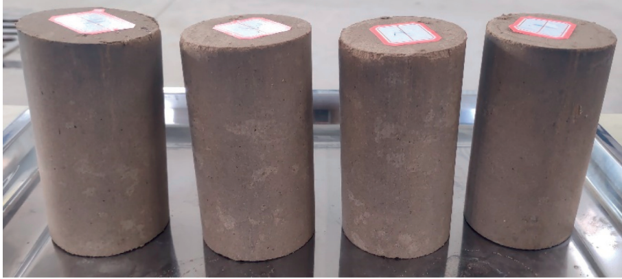
FIGURE 7: Samples for unconfined compression test.
