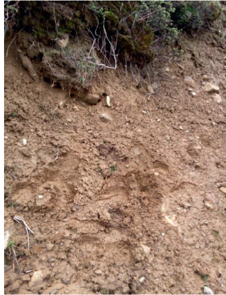
FIGURE 14: Shallow landslide due to multiple freeze-thaw cycles.
