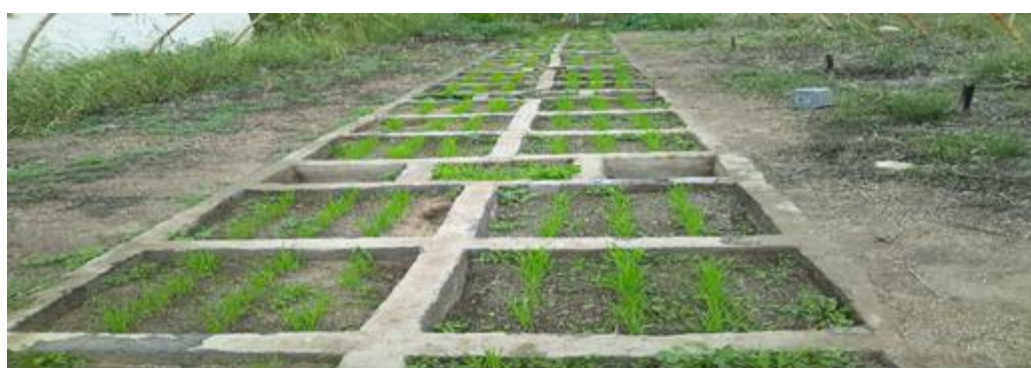
Fig. 1. Lysimeter set used to conduct the experiment
