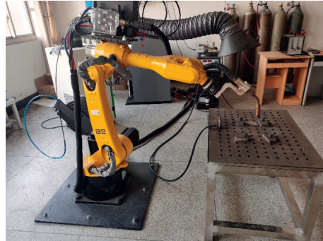
FIGURE 1: WAAM experimental system used in this work.
