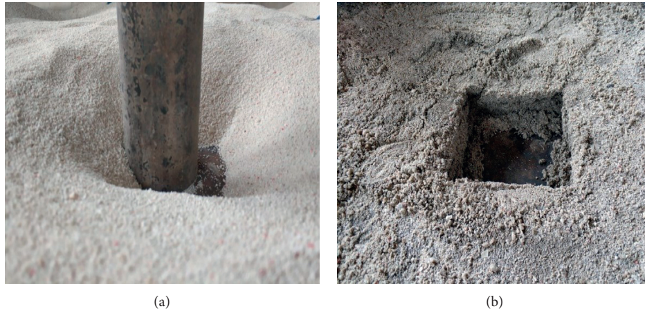
FIGURE 16: Different failure modes of calcareous sand foundation.
