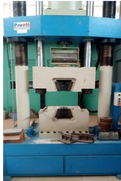
(b) Split concrete cylinder under test
