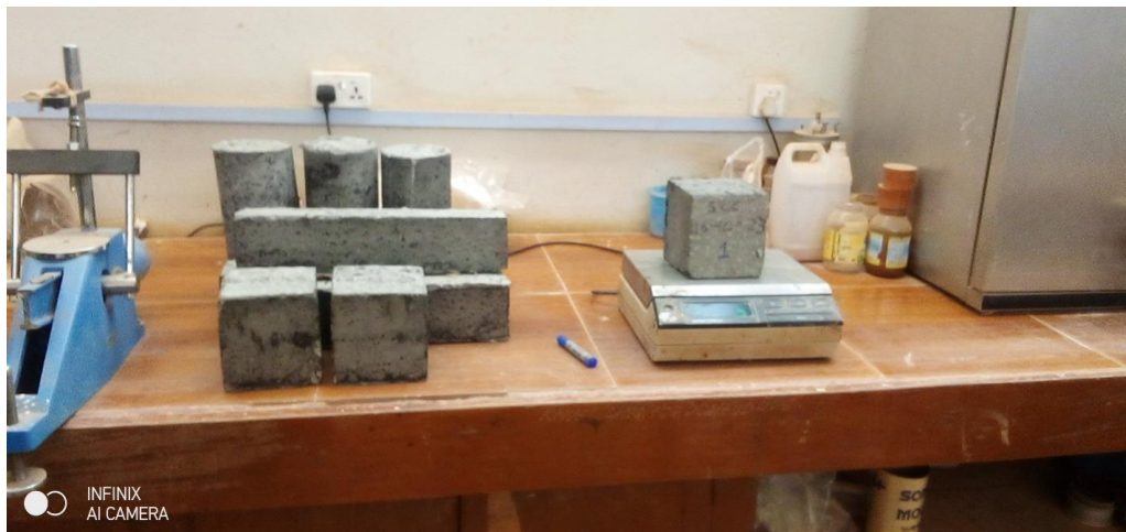
Fig. 2. Concrete test specimens (a) Concrete test cubes, cylinders and Prisms
