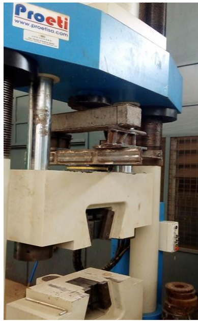
(b) Split concrete cylinder under test
