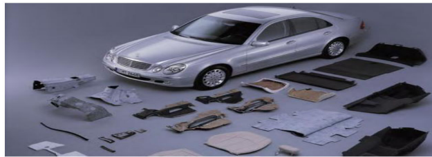
Fig. 3. Mercedes E-class automotive components are made from different bio-fiber reinforced composites (Holbery et al., 2013).
