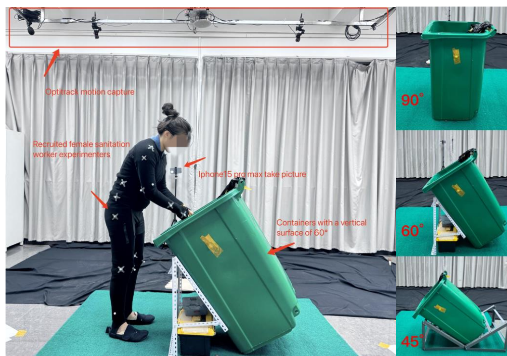
Figure 8. Schematic diagram of experimental setup scene and container inclination angle.
