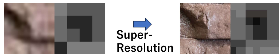
Figure 2. Example of super-resolution of the pair of images of a raw RGB image and its distance image.
