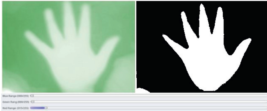
FIGURE 4: Assignment of the threshold for the channel with the colour red and segmented with that information.
