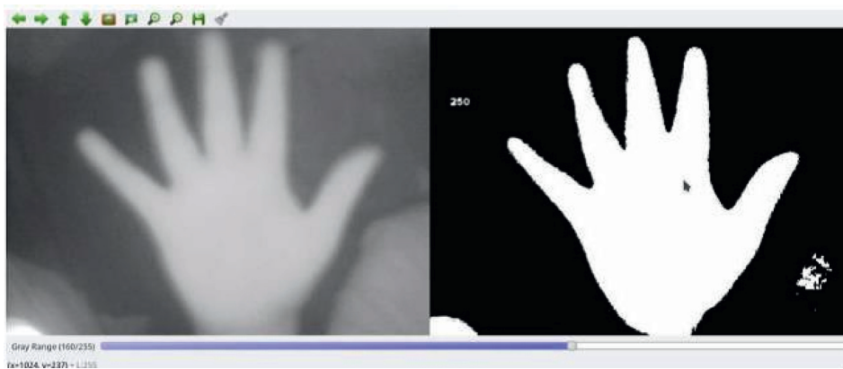
FIGURE 5: Threshold assignment for grayscale and segmented with such information.
