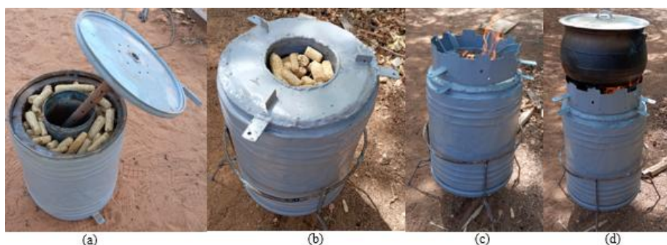
Fig. 4. Principle of use of the multifunctional family oven
