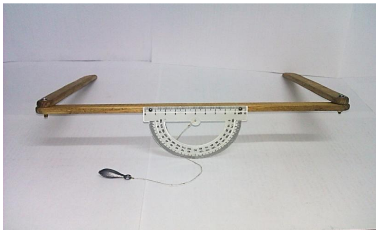
Fig. 2. The pelvic inclinometer used in this study to measure the pelvic inclination angle
