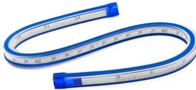
Fig. 1. The flexible ruler used in this study to measure the spinal curves
