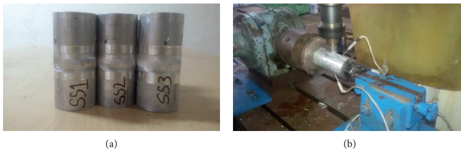
FIGURE 8: (a) Slots made in the piped tube (workpiece). (b) Placement of K-type thermocouple in the FSW setup.
