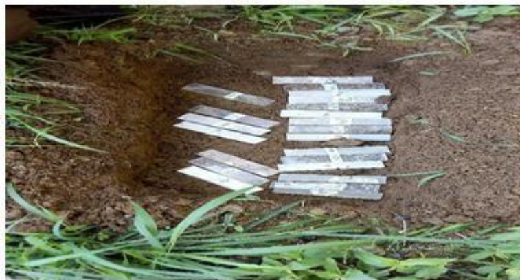
Fig. 4. Burial test (Biodegradability)
