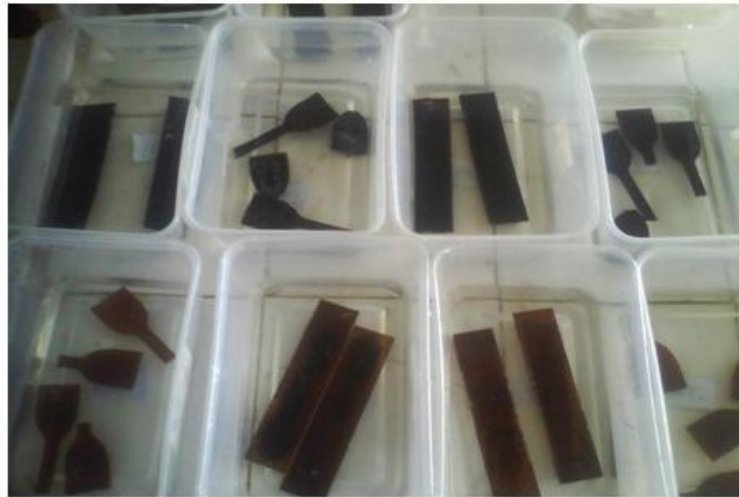
Fig. 3. Water absorption test
