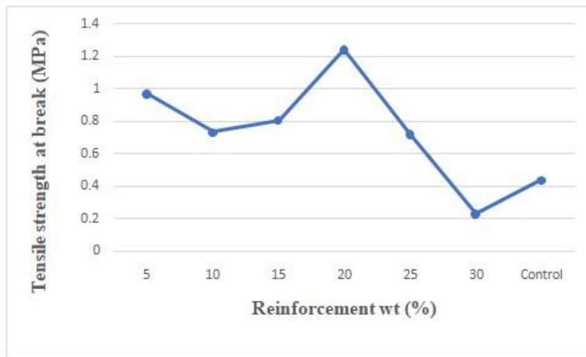
Fig. 6. Variation of tensile strength at break (MPa) with the composite and control
