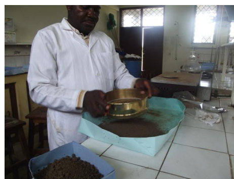
Fig. 3b. Sieving of soil using a 2 mm Sieve
