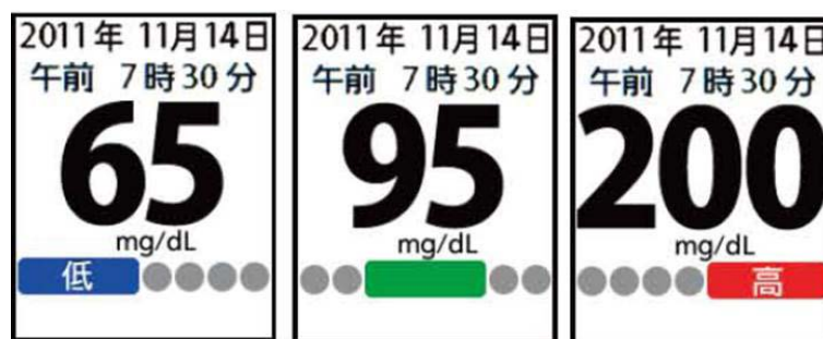
Figure 2. Color range indicator of glucose meter. The first row of the indicator shows year/month/day in Japanese. Second row displays time (hour/minute) in Japanese. Left panel color with kanji character “Low” indicates low blood glucose level with blue-color indicator; middle panel shows normal blood glucose level with green-color indicator; and right panel shows high blood glucose level with red-color with kanji character “High”.
