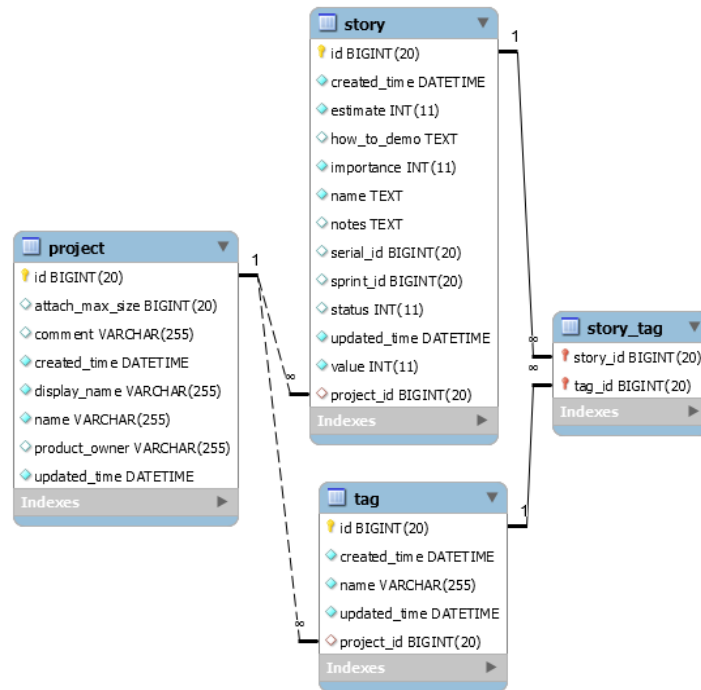
Fig. 8. Entity relationship diagram of product backlog microservice table
