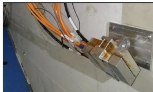
Figure 3. Timepix3 (TPX3) hodoscope using two TPX3 sensors, operated at LHC Run-2. The device was mounted in the ATLAS experiment cavern at CERN.
